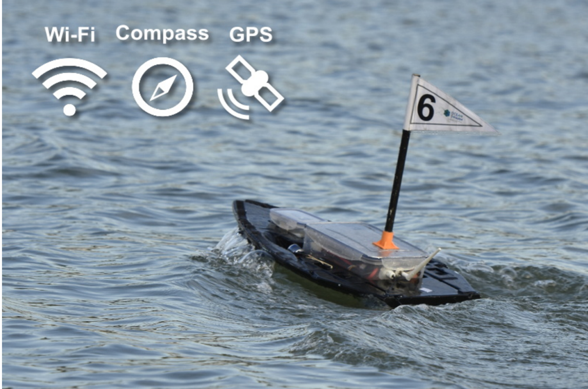
Figure 1.12: Surface Boat Equipped With a Compass, GPS, IMU for Studying the Performance of a Over Surface Robots in a Real Aquatic Environment for Achieving a Collective Goal Such As Clustering, Homing.
