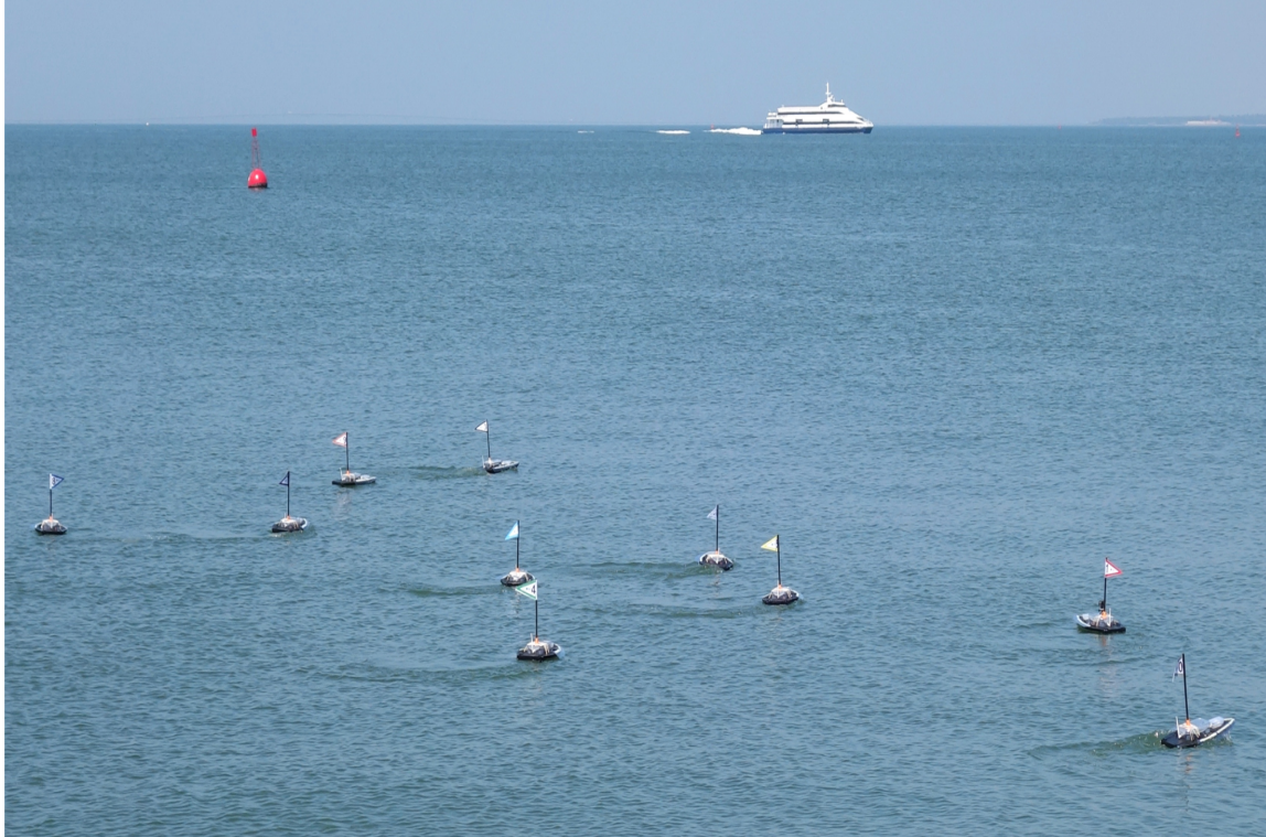
Figure 1.13: Swarm of 10 Boats Used to Study the Performance of Swarming Strategies in a Real World Aquatic Environment.
