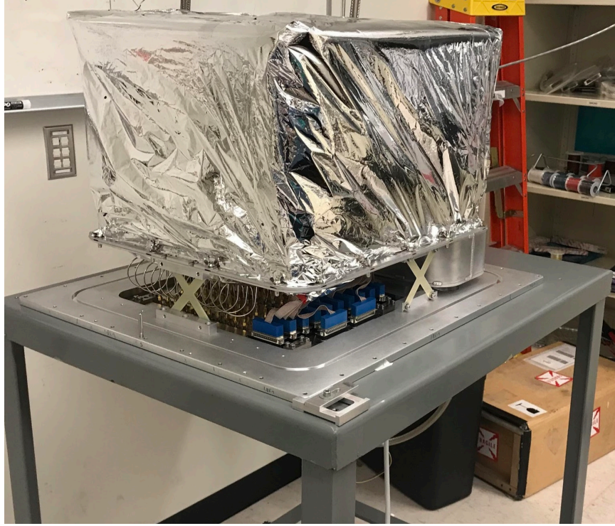
Figure 33. Radiation shields cover the 40K and 4K stages of the harness test cryostat
