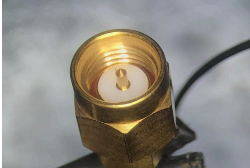
Figure 30. A faulty SMA connector. Excess dielectric material protrudes beyond the metal contact ring and prevents proper mating.
