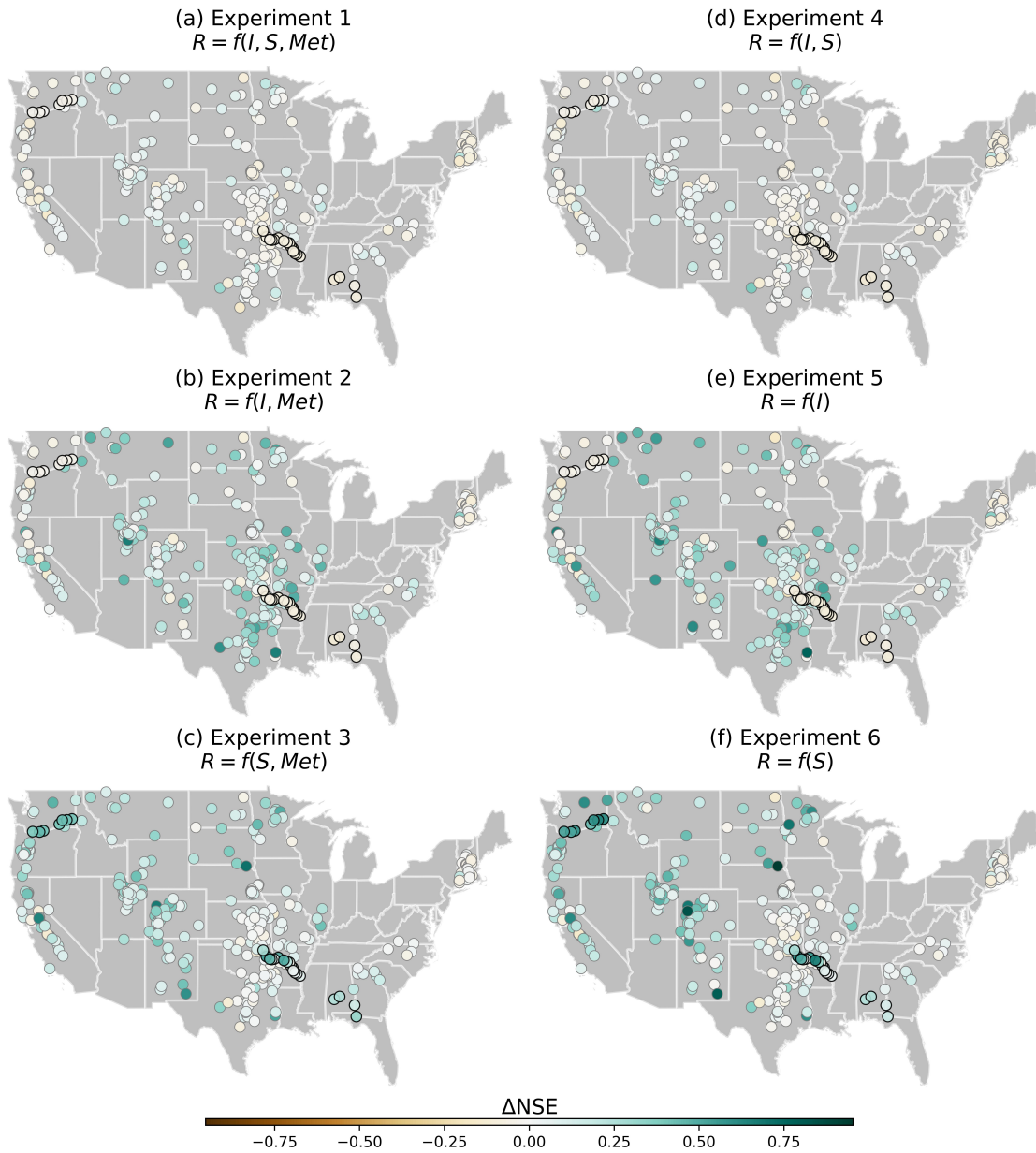
Figure 2.4: Spatial distribution of average Nash-Sutcliffe Efficiency (NSE) improvement \Delta NSE from Daily scale to hierarchical time scale configuration of Data-driven models in (a) Experiment 1, (b) Experiment 2, (c) Experiment 3, (d) Experiment 4, (e) Experiment 5, and (f) Experiment 6. The circles with black solid edges represent reservoirs labeled as “lock and dam.”
