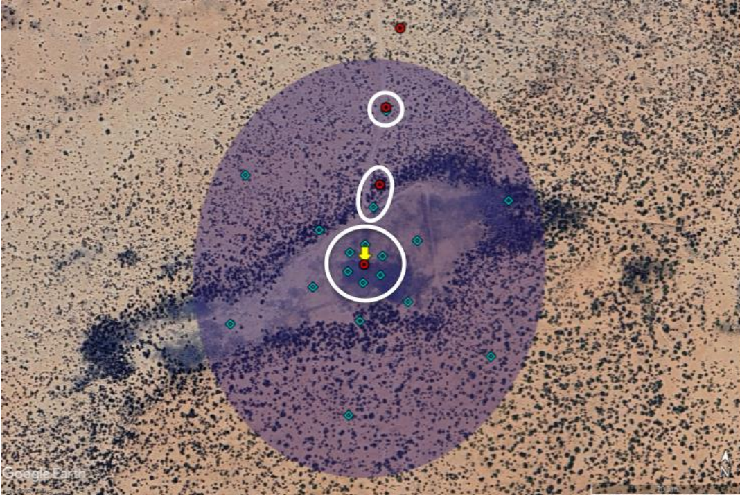
Figure 20. Sample Map of the Small Playa Site. The sampling coordinates (teal diamonds) from Hurtado et al., 2024 sit on top of the same map from Figure 16 (yellow arrow points to the location of COSMOS, blue region the COSMOS footprint, and the red dots are RV stations). Note that several of these sites are within a few meters of the RV stations along the RV traverse. Samples were collected at radii of: 25 m, 75 m, and 200 m. For each RV station, the closest sample(s) was used as ground truth (white circles). For the station closest to COSMOS, the samples along 25 m radius circle were averaged. For the 100 m station, the nearest 75 m sample was used. For the 200 m station, the nearest 200 m sample was used. Since no samples were collected beyond the 200 m station, the 300 m station was compared to the 200 m sample.
