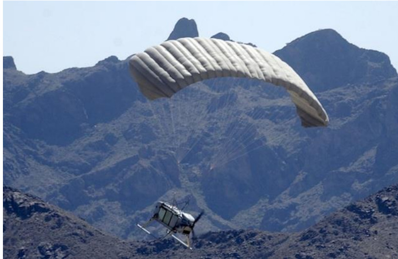
Figure 2: The CQ-10 Snowgoose PPC UAV for Heavy Lift
