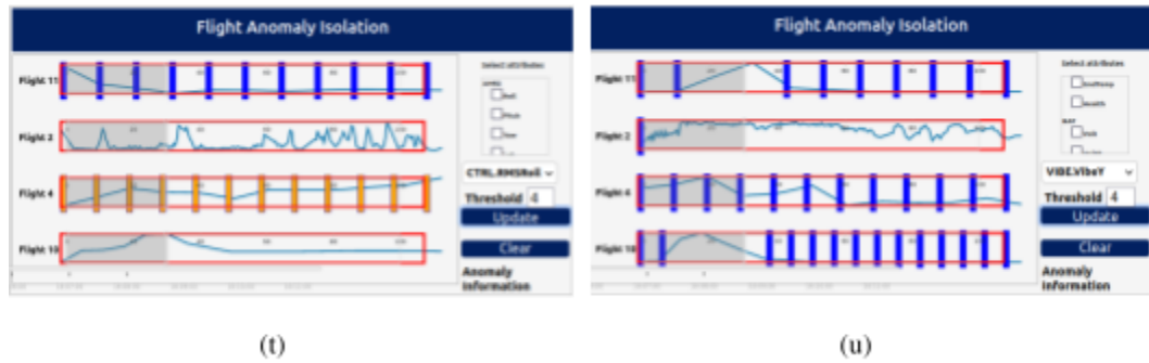
Figure 5.14: (t) CTRL stands for Attitude Control oscillation monitor diagnostics, and RMSRollP is LPF Root-Mean-Squared Roll Rate controller P gain. (u) VIBE stands for processed (acceleration) vibration information, and VibeY occurs on the y-axis.
