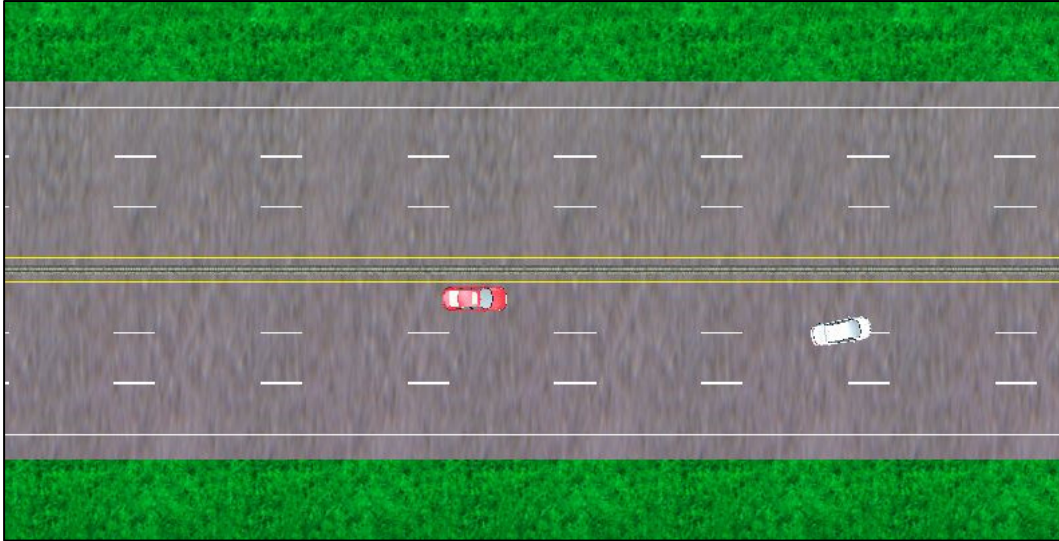
Figure 36. Cut-In Scenario Setup in HVE Illustrating Lead Vehicle (White) Changing Lanes in Front of Follow Vehicle (Red)
