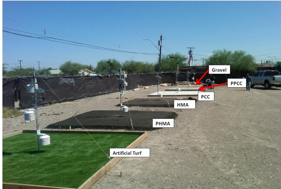
Figure 8 – Full-Scale Pavement Test Slabs in Tempe, Arizona
