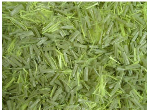
Figure 106 Fiber blend incorporated into the Evergreen Drive mixture (Kaloush et al, 2008).
