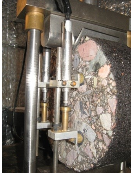
Figure 91 Vertical LVDT's mounted on CFT specimen
