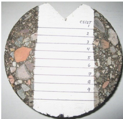
Figure 6 – Final C* fracture test specimen.
