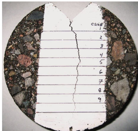
Figure 30 Crack visibility using white paint.
