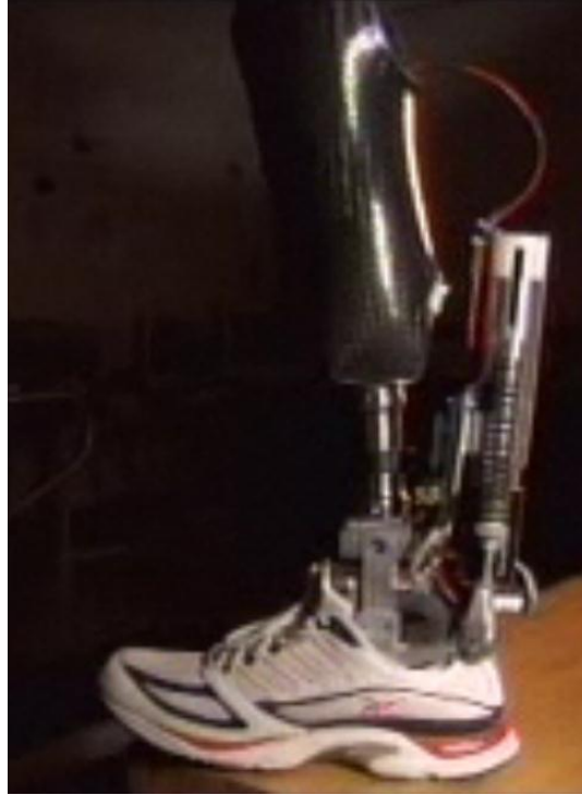
Figure 1: SPARKY. Spring Ankle with Regenerative Kinetics.
