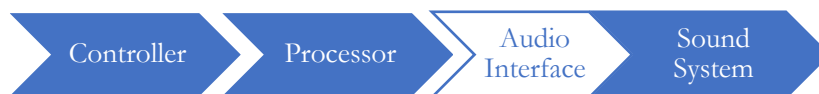
Figure 6. Graphic Demonstrating the Flow of Equipment When an Audio Interface Is Incorporated.
