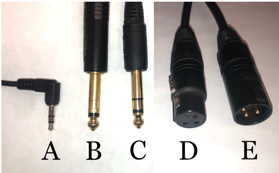
Figure 1. Common Audio Connectors Seen in Electronics Setups. From Left to Right: 1/8" TRS Male (A); 1/4" TS Male (B), 1/4" TRS Male (C); XLR Female (D); XLR Male (E).
