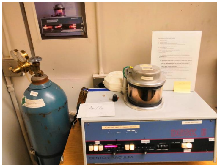
Sputtering: Au/Pd sputtering tool used to coat sample before SEM analysis.
