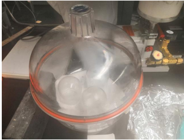
Epoxy encapsulation: Vacuum oven setup to for epoxy curing preparation
