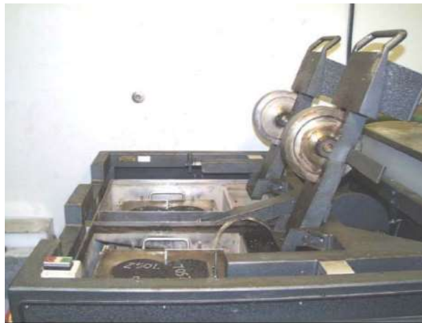
Figure A-17. Hamburg wheel tracking device (Texas Transportation Institute 2007).
