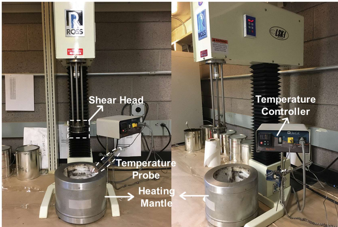
Figure A-20. High Shear Mixer and its Components Used for the Binder Preparation.
