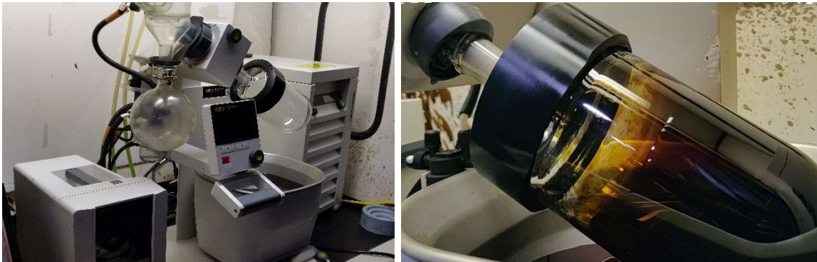
Figure 5-5 Binder Recovery: (a) RotoVap Setup; and (b) Binder Flask Immersed in the Hot Oil Bath
