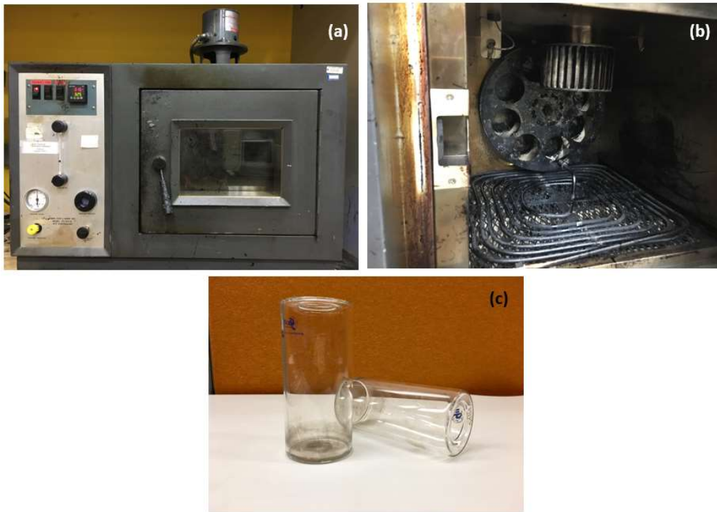
Figure A-1. (a) Overview of RTFO, (b) Inside the RTFO, and (c) RTFO Bottle.
