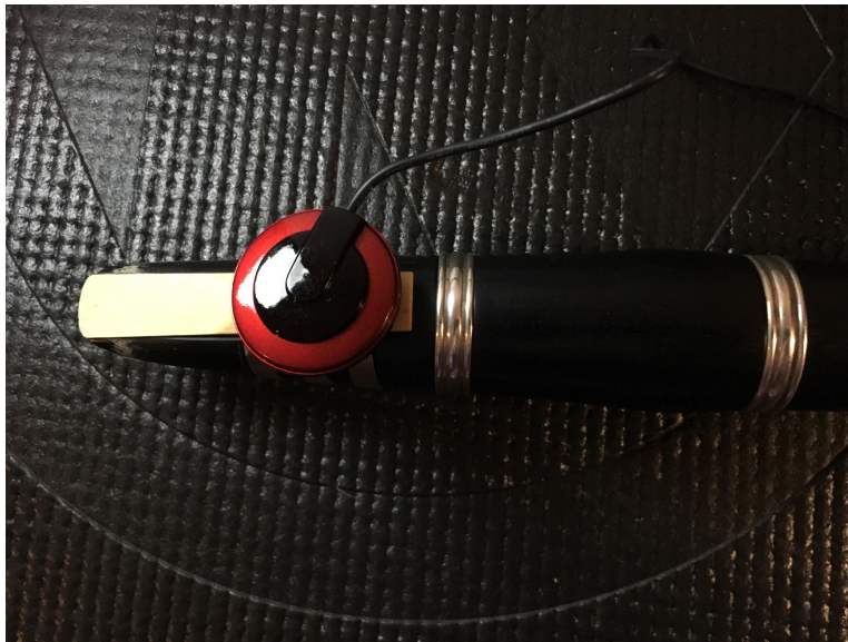
Figure 5.1: Ligature (LIG) placement of contact pickup.
