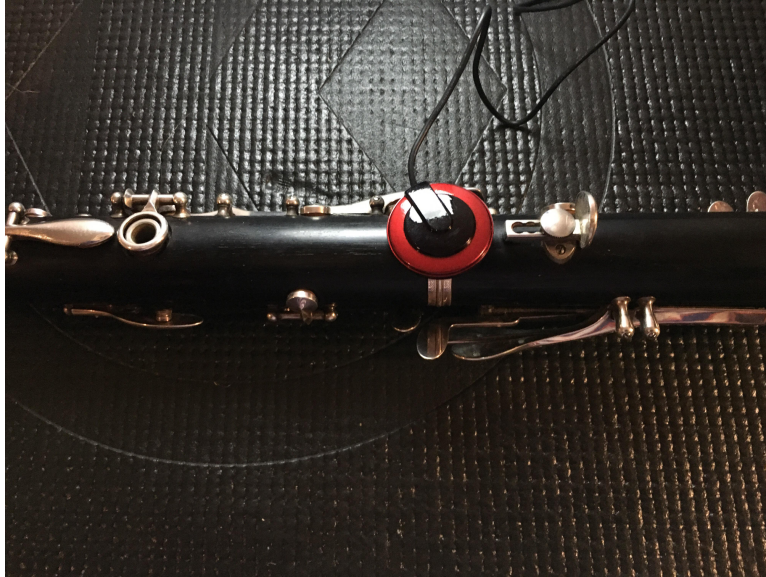
Figure 5.8: Center tenon (CTR) placement of contact pickup.
