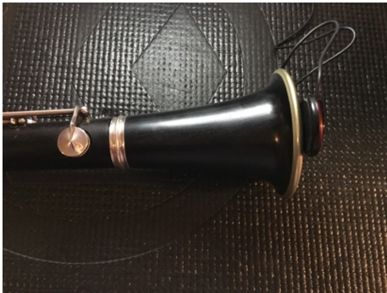
Figure 5.11: End of bell (BELL End) placement of contact pickup. Note placement perpendicular to bore.
