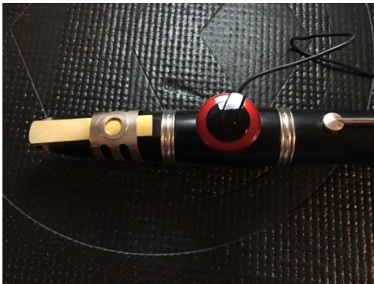
Figure 5.3: Barrel surface (BAR Surf) placement of contact pickup.
