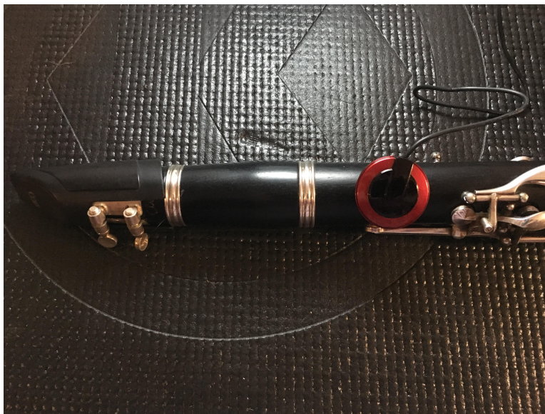
Figure 5.7: Upper joint (UJ) placement of contact pickup.
