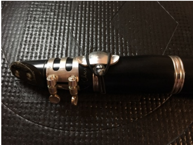
Figure 5.5: LefreQue plates spanning the mouthpiece and barrel joint (LF MPB). Pickup was placed directly on the bridge.
