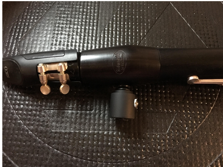
Figure A.1: Nalbantov NCM 8X barrel pickup with included barrel.
