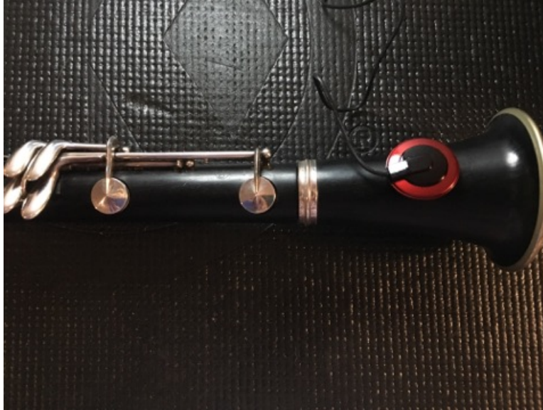
Figure 5.10: Outside of bell (BELL Out) placement of contact pickup.
