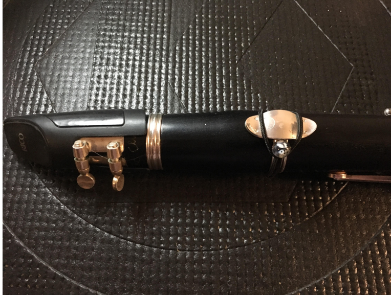
Figure 5.6: LefreQue plates spanning the barrel and upper joint tenon (LF BUJ). Pickup was placed directly on the bridge.
