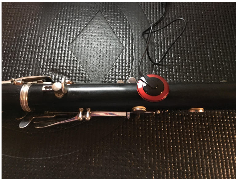
Figure 5.9: Lower joint (LJ) placement of contact pickup.
