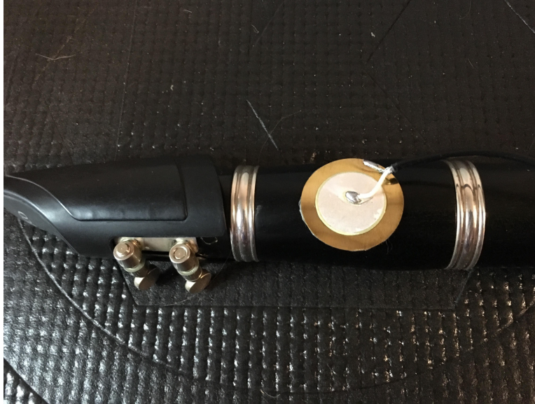
Figure 5.4: Barrel surface placement of contact pickup with plastic cover removed (BAR NC)
