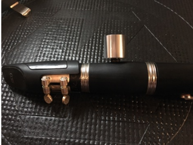
Figure 5.2: Ported barrel pickup (BAR Port) by PiezoBarrel.
