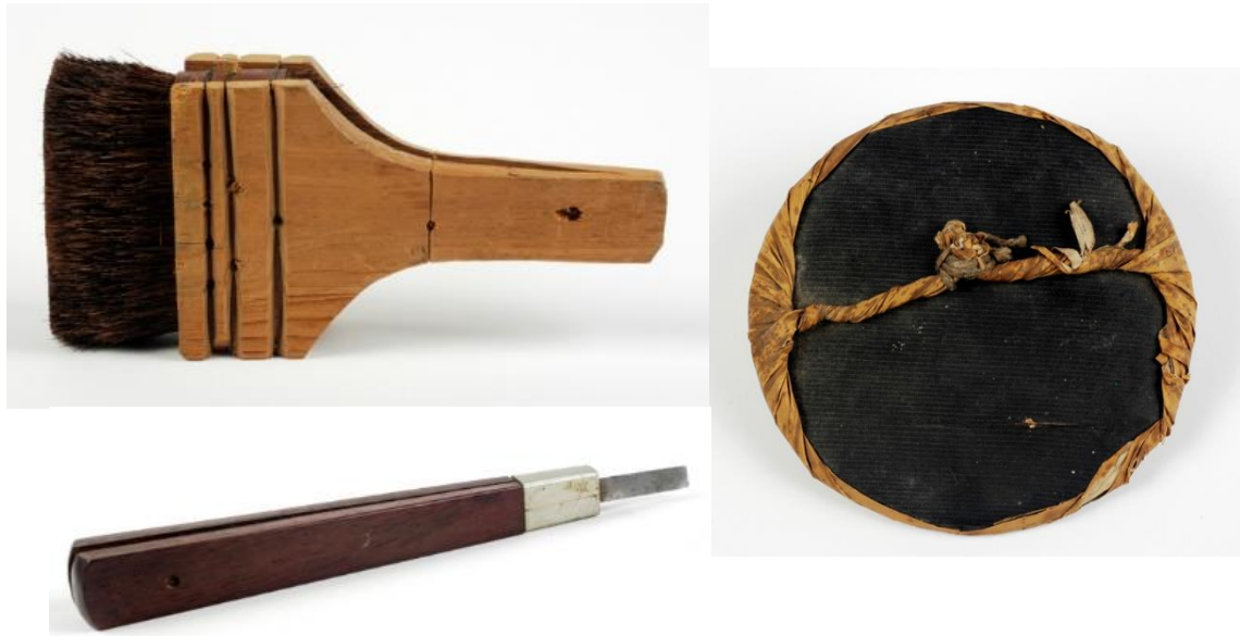
Figure 3.21: A Selection of Helen Hyde's tools including, flat brush ( top left ), carving tool ( bottom left ) and baren ( right ). Brush: 15.2 x 3.5cm; Carving tool: 11.75 x 1 x 1 cm; Baren: 12.7 cm (diameter). Jordan Schnitzer Museum of Art. Gift of Dr. Don E. and Carol Steichen Dumond, 2003. Source: Photos Courtesy of the Jordan Schnitzer Museum of Art.
