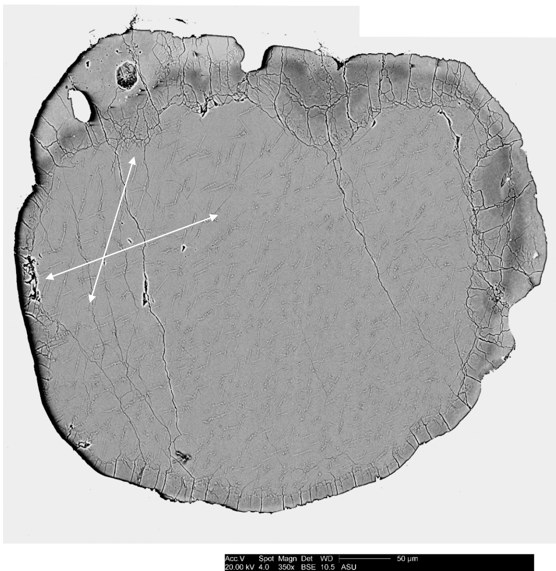
Fig. 3.12. BSE Image of Sample BB755A (~75 ppmw; 900 °C; 7 hrs.). Intracrystalline lenses of ringwoodite/wadsleyite tend to nucleate along preferred orientations (indicated by arrows).
