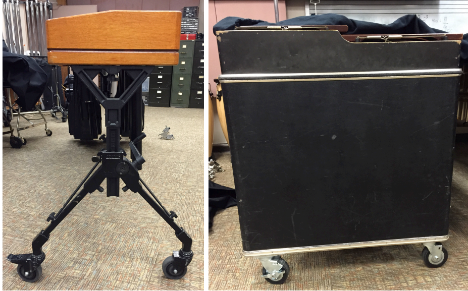
Figure 2.1: Both types of standard marimba frame ends. Left to right, Adams Artist 5.0 octave high end, Musser 4.3 Octave low end.
