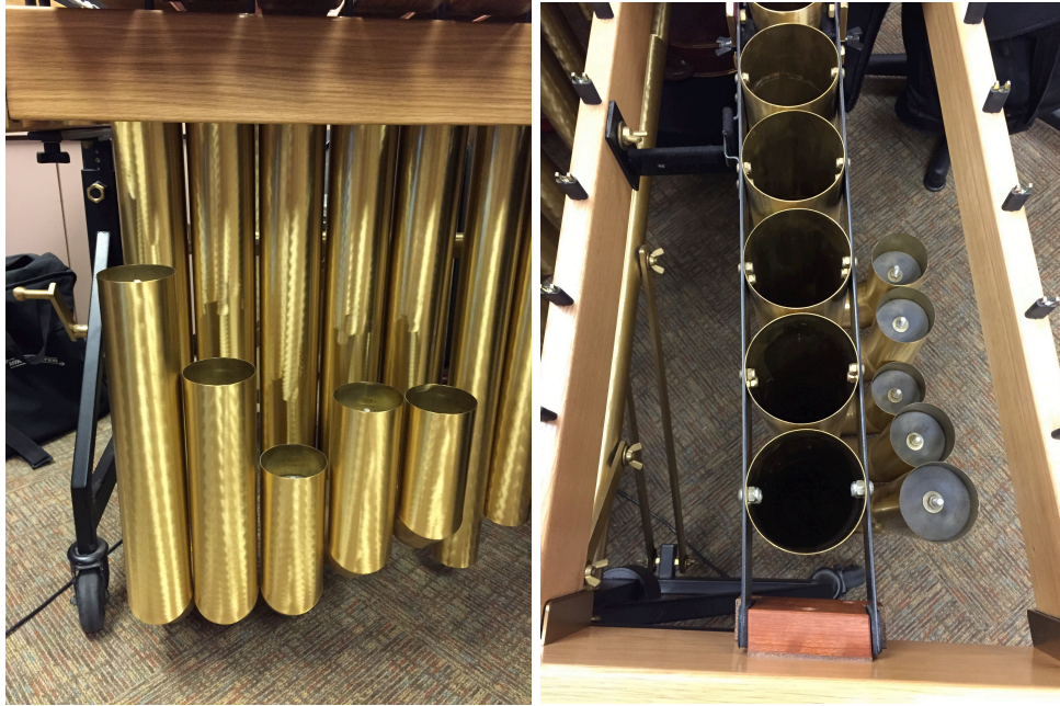
Figure 2.2: Side and upper view of tubular resonators (Pictured, Demorrow M5 Concert Marimba).
