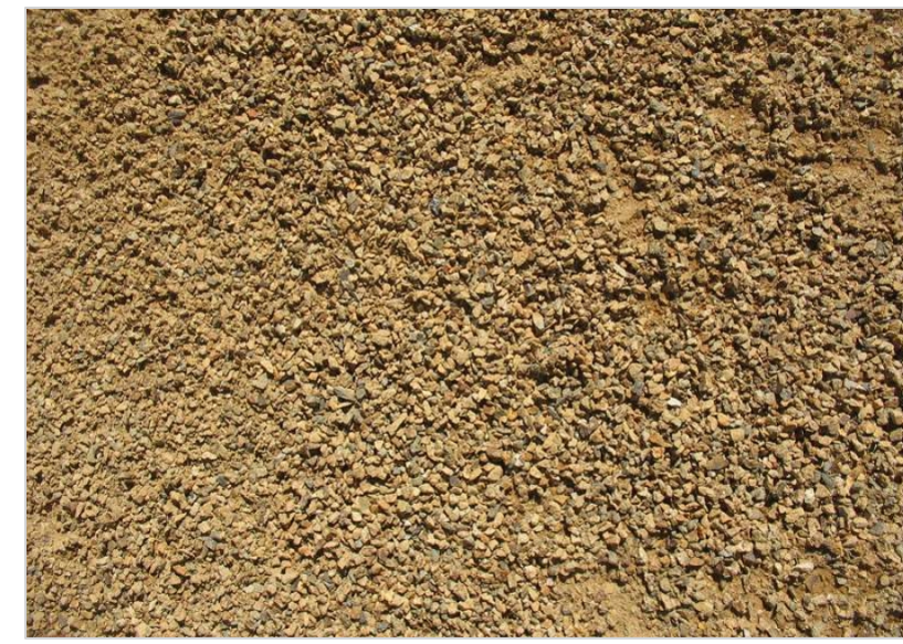
Figure 2-7: Crushed Rock with Fines (ParsonsRocks.com)
