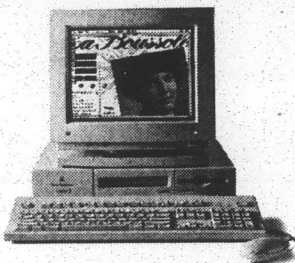
Power Macintosh® 6100/66 w/CD 8MB RAM/350MB hard drive, CD-ROM drive, color display, keyboard and mouse.
