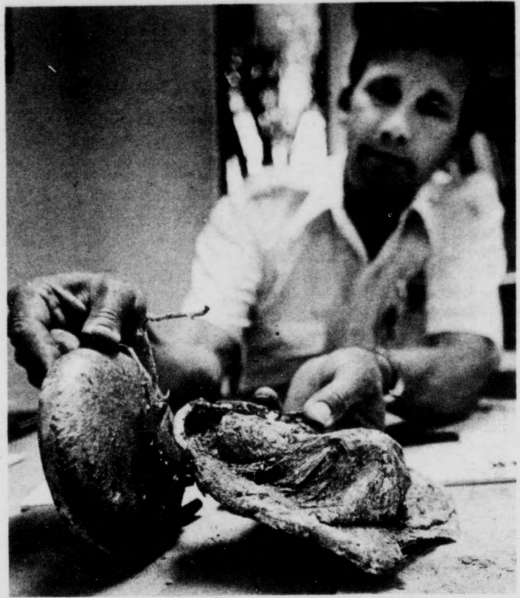
Fire Marshal Sylvester Anderson holds the melted remains of a wall lamp that caused Tuesday's fire in Neeb Hall. Anderson said $15,000 damage was done to the building. [State Press staff photo]
