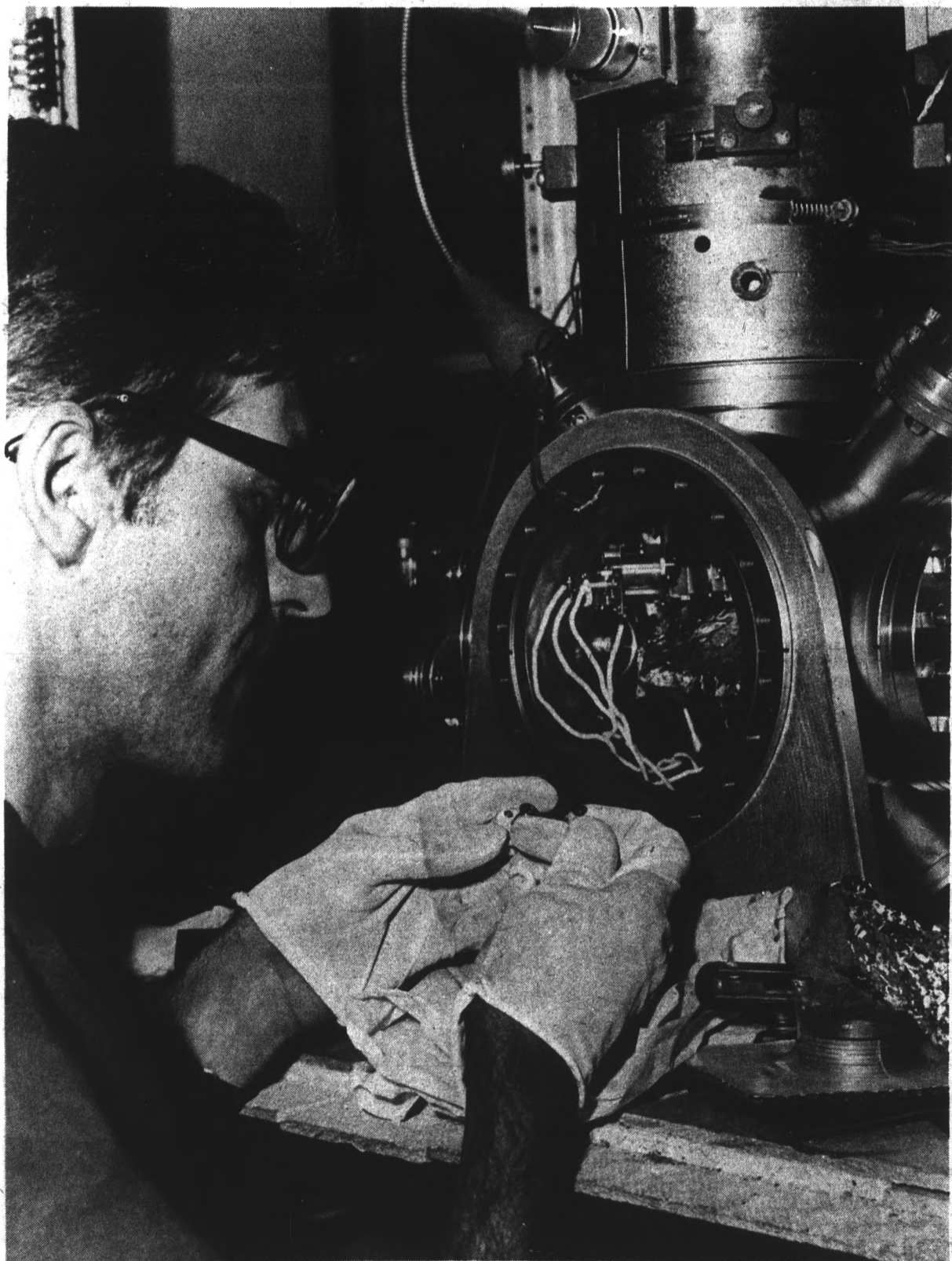
A gold crystal is loaded into a new high vacuum electron microscope by Dr. Dave Landry of ASU's Center for Solid State Science. The experimental instrument has to be partially disassembled to load the specimen because of heavy insulation for the vacuum. The device studies the arrangement of atoms on the surface of crystals to determine how crystals undergo chemical reactions.
