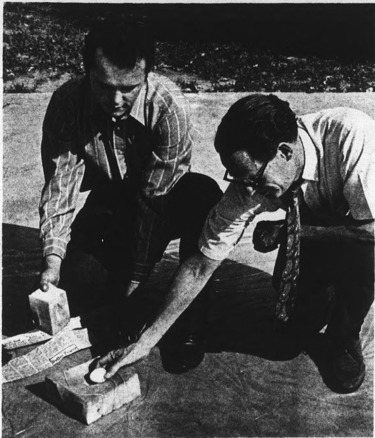
IMPOSSIBLE PROBLEM? — A foam rubber cushion was the successful answer to one egg-packaging problem posed to freshmen mechanical engineering students. Tommy Thompson and Dr. Ernest Chilton inspect the package after it was lowered from a 12-foot ladder.
