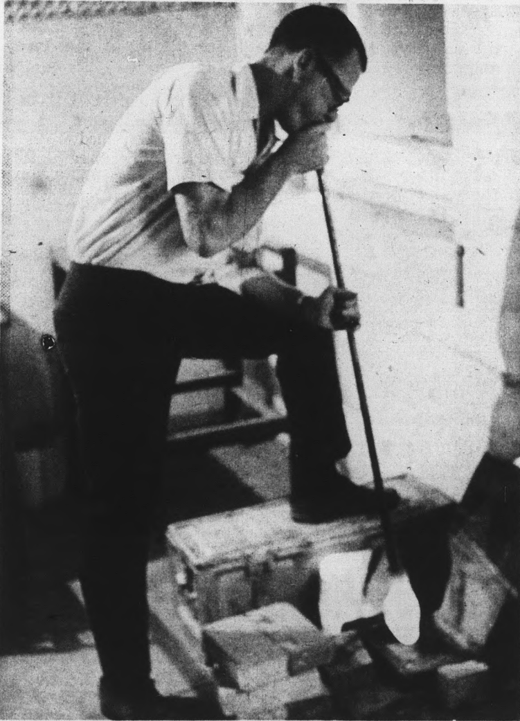
MIRROR OF CREATION — Prof. Henry Schrieber watches the process of creation in a mirror as he shapes a molten blob of white-hot glass with his breath.
