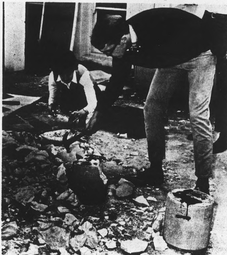
FINALLY — After the metal has solidified, the mold is chipped away, leaving a rough, unfinished cast.
