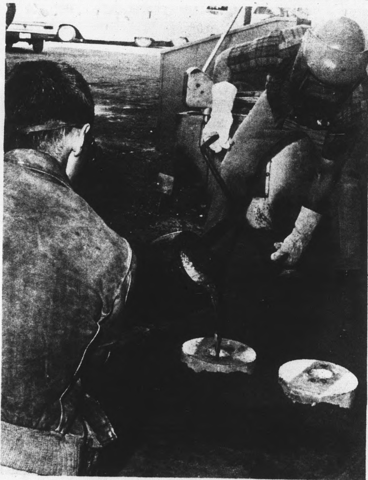
POURING THE METAL — Molten bronze is poured into the silt-packed molds. Smaller holes appearing on top of the mold are vents which allow rapidly expanding gases to escape. The vents, connected to the cast itself, are also filled with molten bronze. After the metal solidifies and the mold is removed, the vents and sprues, also filled with bronze, protrude from the cast in all directions. They will be cut off before the cast is finished and polished.
