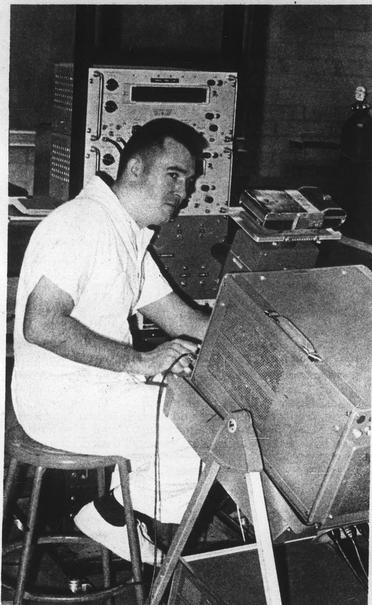
SHOCK TUBE — Graduate student L. B. Haws works the controls of Prof. Donovan Evans' newly designed shock tube. The instrument is used to test high velocity and its effects at different pressures.
