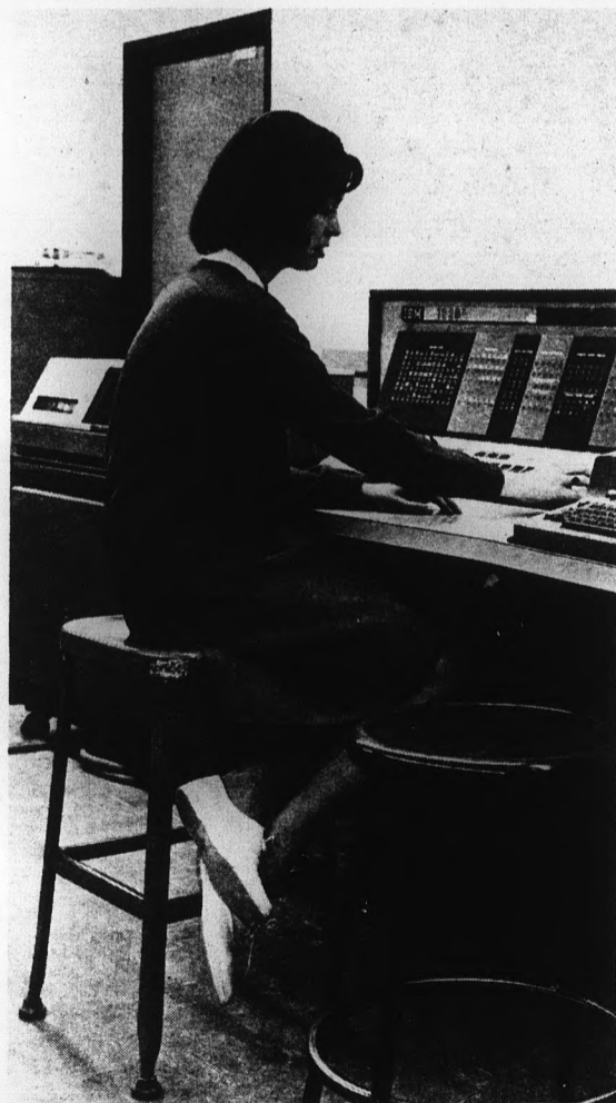
Linda Germroth operates the 1620 IBM Consul, the main control panel that feeds information to tape decks or 'memory banks.' Visible behind her is disc pack unit that contains 2 million 'bits' of information and that makes computer operations nearly automatic.
