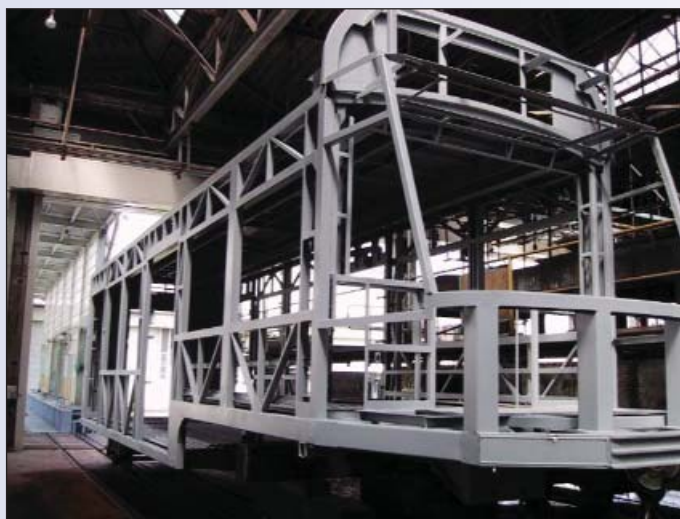
METRO vehicle prototype in the early manufacturing phase at the Kinkisharyo plant in Osaka, Japan
