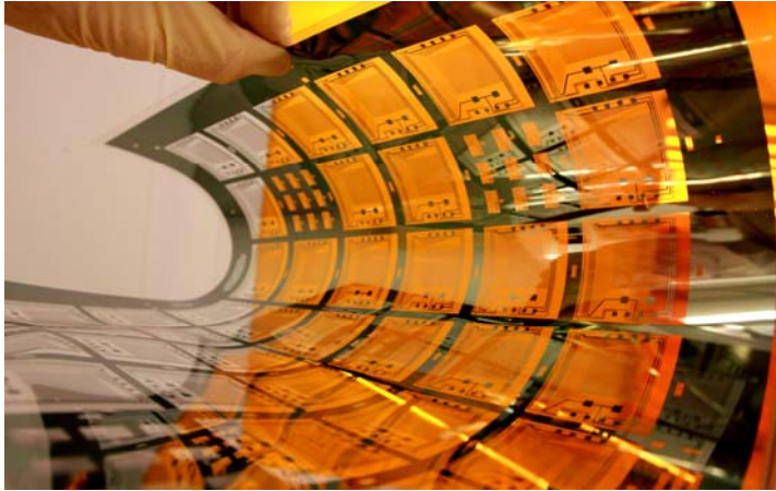
Printable, plastics based flexible display developed by interdisciplinary Advanced Materials researchers at ASU
