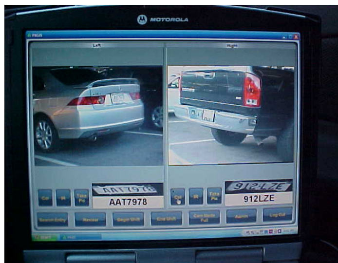
Demonstration screen viewed by officers in the vehicle when utilizing an Automated License Plate Reader
