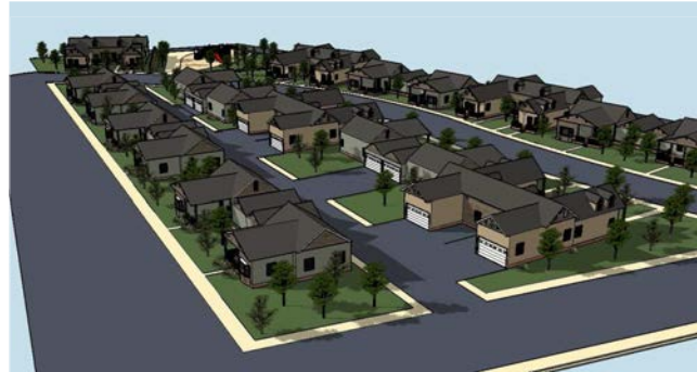
Figure 24: Alley Loaded Attached Single-Family Homes
