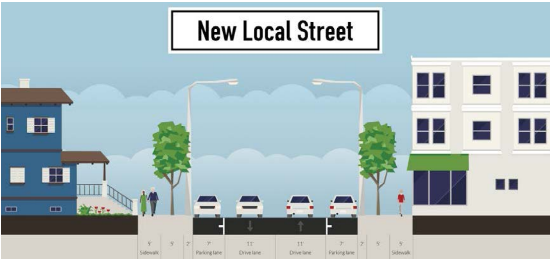
Figure 20: Cross-Section of New Local Street (60-foot right-of-way)
