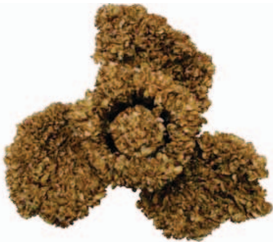
A propeller infested with quagga mussels.
