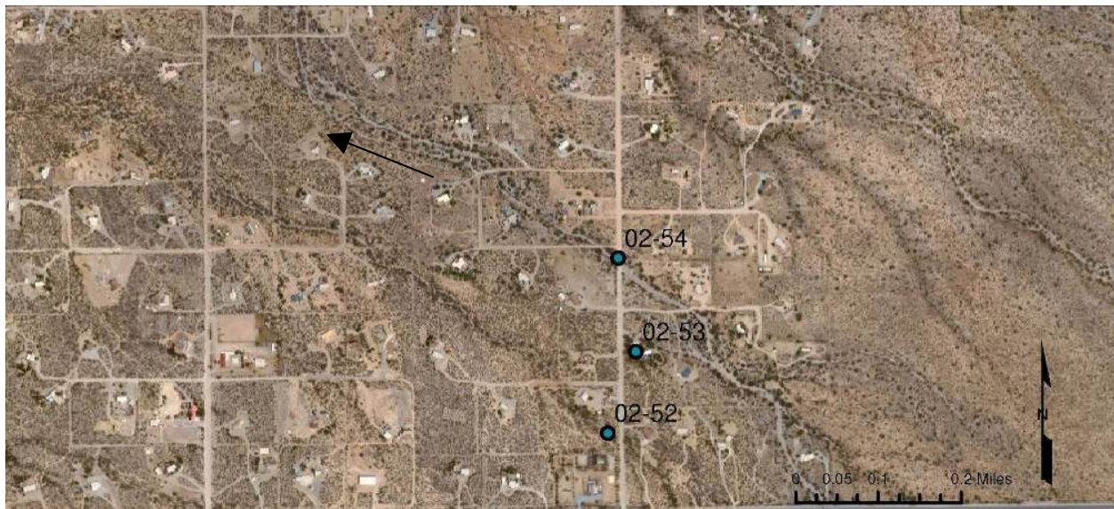
Aerial view of headcutting washes crossing Salero View Road
