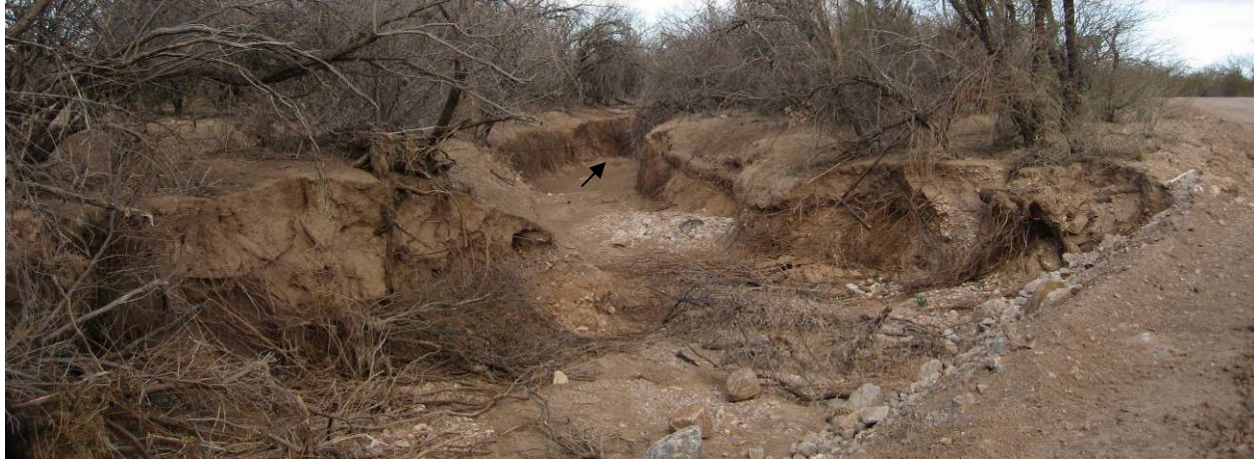
Vertical banks and scour downstream of Old Nogales Highway on Petty Ranch Wash, T2 surface (LM04-02-03)
