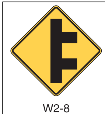
Figure 34: Double Side Road Intersection Warning Sign
