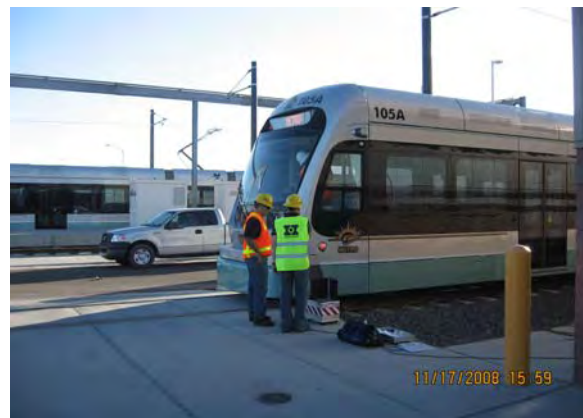
LRV Train to Wayside Communications Testing
