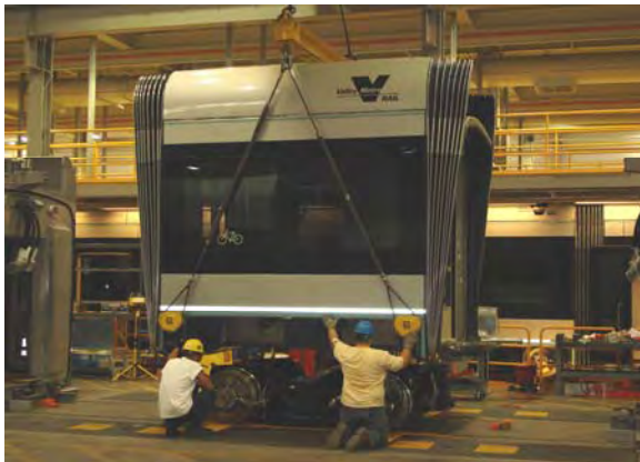
Car C section being prepped for final assembly
