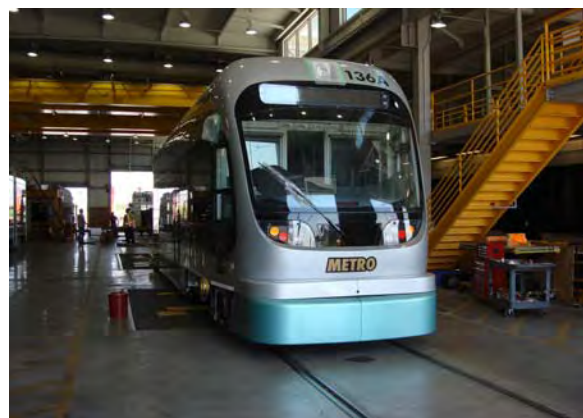
Car articulated and prepping for static testing
