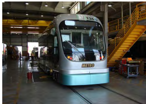
Car articulated and prepping for static testing
