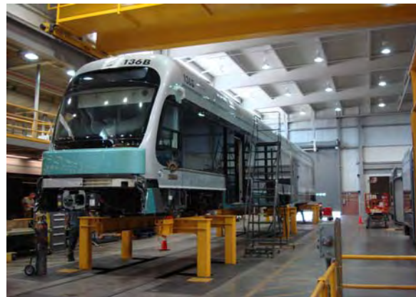
Car under floor work
