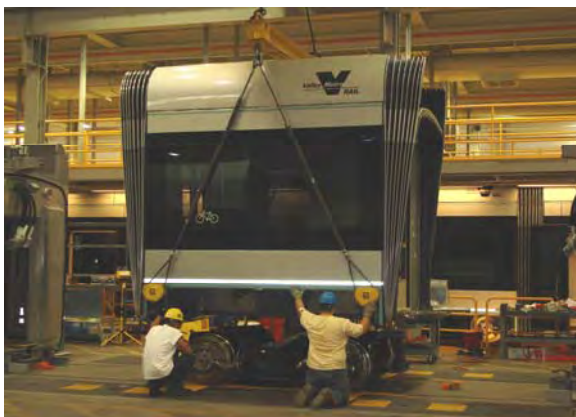
Car C section being prepped for final assembly
