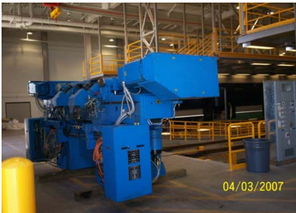
Wheel Profiling Machine ready for installation
