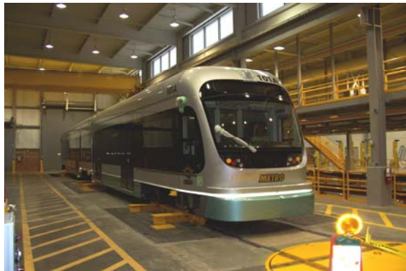
Car 101 being used to test the LRV car hoist
