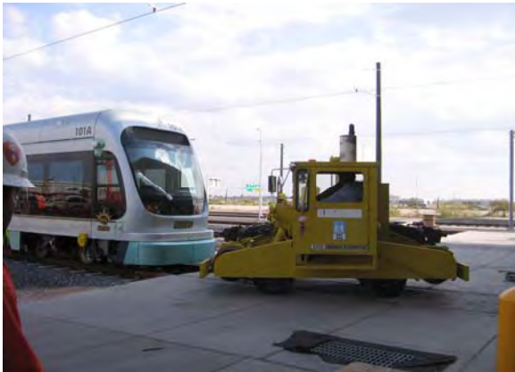
LRV 101 movement for testing of hoist and lift equipment at OMC.
