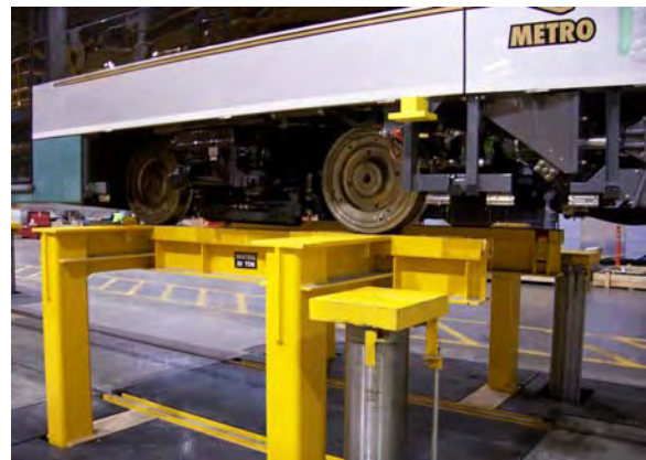
Car 101 on the new LRV car hoist
