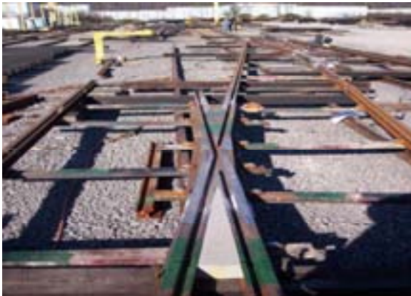
First Article inspection photos of a right hand crossover for Line Section 4 at the contractor's facility in Birmingham, Alabama.
