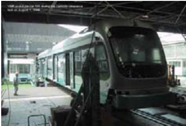
Carbody clearance test. Prototype car 101, August 1, 2006.
