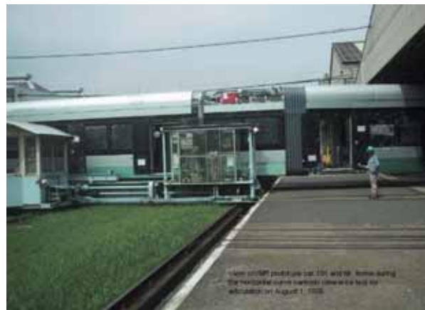
Horizontal curve carbody clearance test for articulation. Prototype car 101, August 1, 2006
