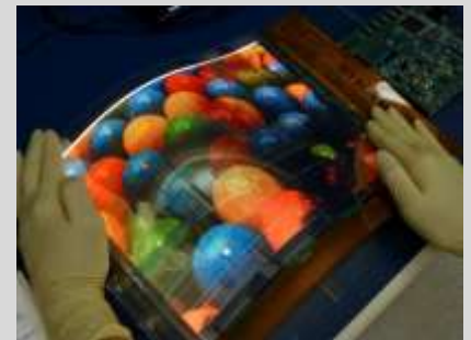
In 2013, FEDC designed and manufactured the world's largest flexible X-ray detector and the world's largest flexible color organic light emitting display.
