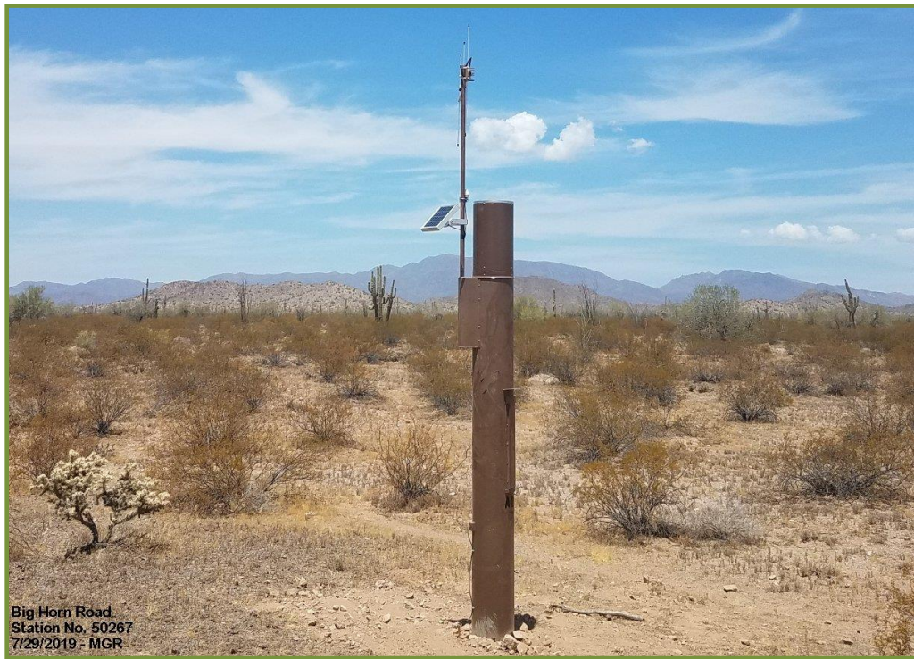
Big Horn Road Rain Gage, Station 50267, Installed 07/29/2019
