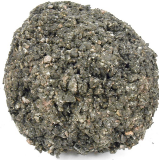
Figure 4. Aged Cantabro Specimen after Testing
